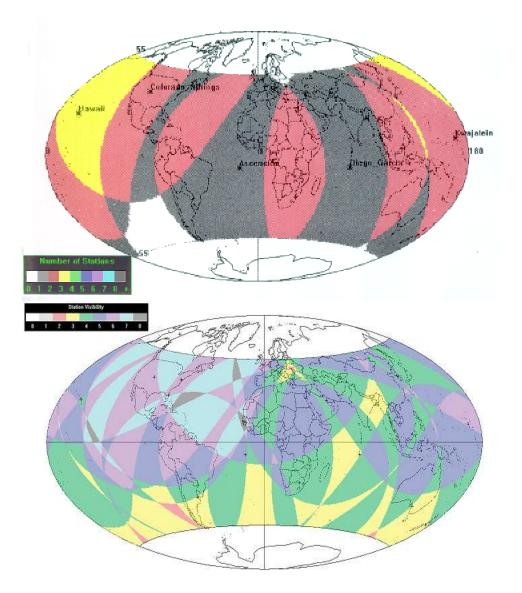
Figure 2. NGA Monitor Stations (MS) impact on GPA satellite visibility: (top) Satellite visibility by ground based AF MS and (bottom) Satellite visibility by combined AF and NGA MS network. (Visibility Legend Information: White: 0 MS, Dark Gray: 1 MS, Salmon: 2 MS, Yellow: 3 MS, Green: 4 MS, Blue: 5 MS, Violet 6 MS, Cyan 7 MS, and Light Gray 8 MS)
